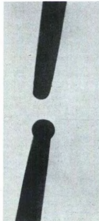
Fig. 2 (a)—The burnt-out tungsten filament of a 4220Z water-cooled valve. (b) An enlarged view of the burnt-out filament.
